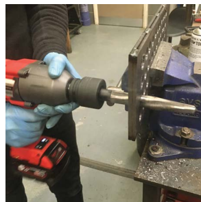
Hex head for use with 1/2" or 3/4" drive hex socket
