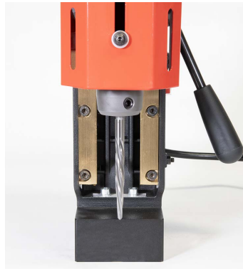
3/4" Weldon Shank for use in magnetic drill
